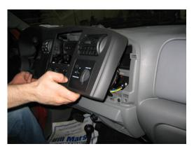
Remove enough to expose hex screws holding lower portion of dashboard
